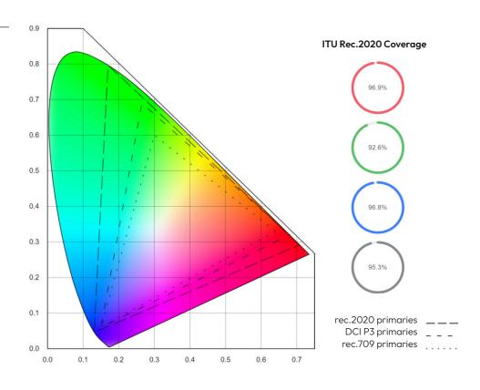
**CIE xy Chromaticity Diagram** Megapixel proprietary LED package gamut shown
