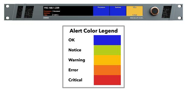
Figure 39: OMNIS front panel alert
