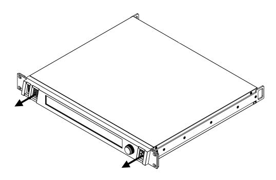
Figure 45: Remove air intake filters for service.
