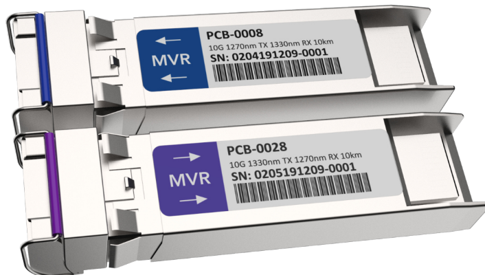
Figure 150: Send and receive SFP+ units.
